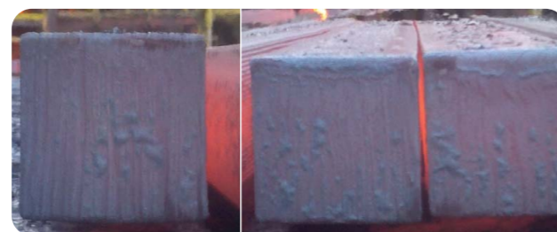
WAVE Mould billet (left) with excellent shape compared to standard mould billets (right)
