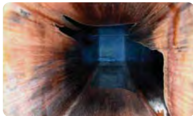
Severe and non-uniform mould wear associated with billet rhomboidity
