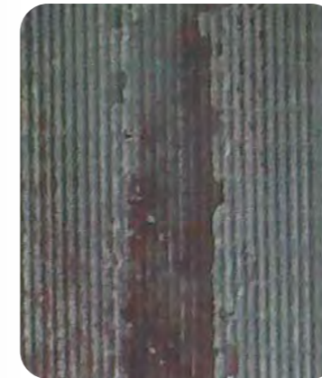
Well-formed pattern on billet cast with WAVE Mould
