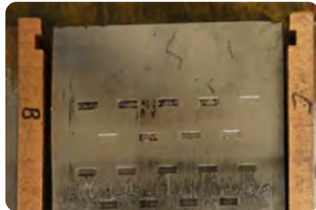
Fig. 8: Meniscus of moulds after 1500 heats
