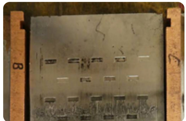
Fig. 8: Meniscus of moulds after 1500 heats
