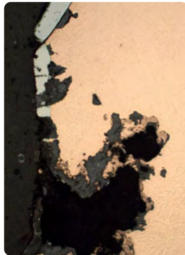
Black spots are sulphur corrosion
