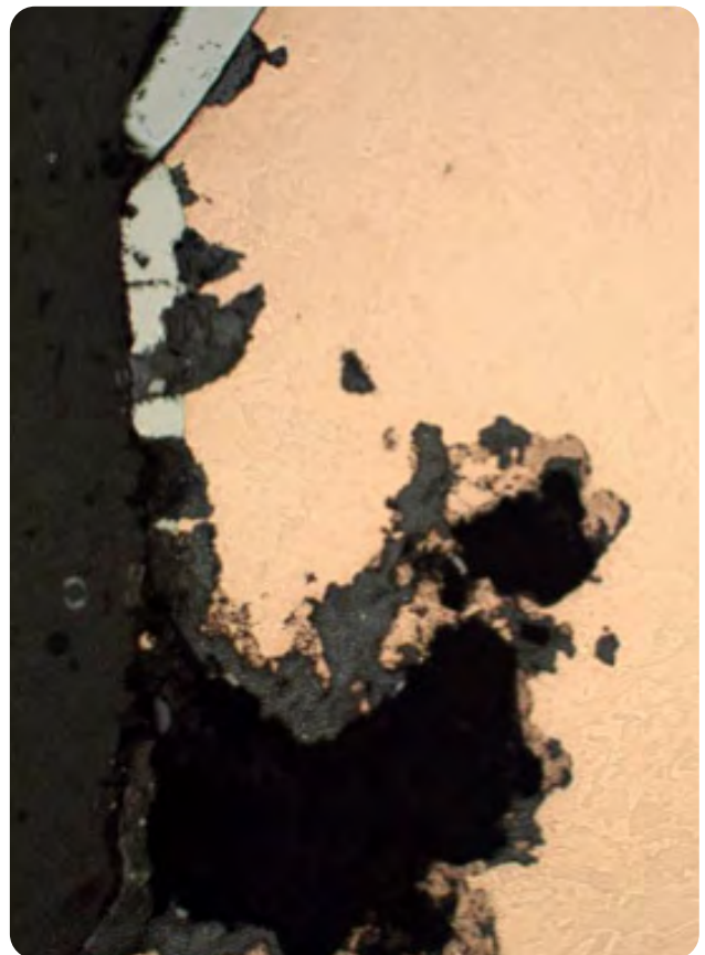
Black spots are sulphur corrosion
