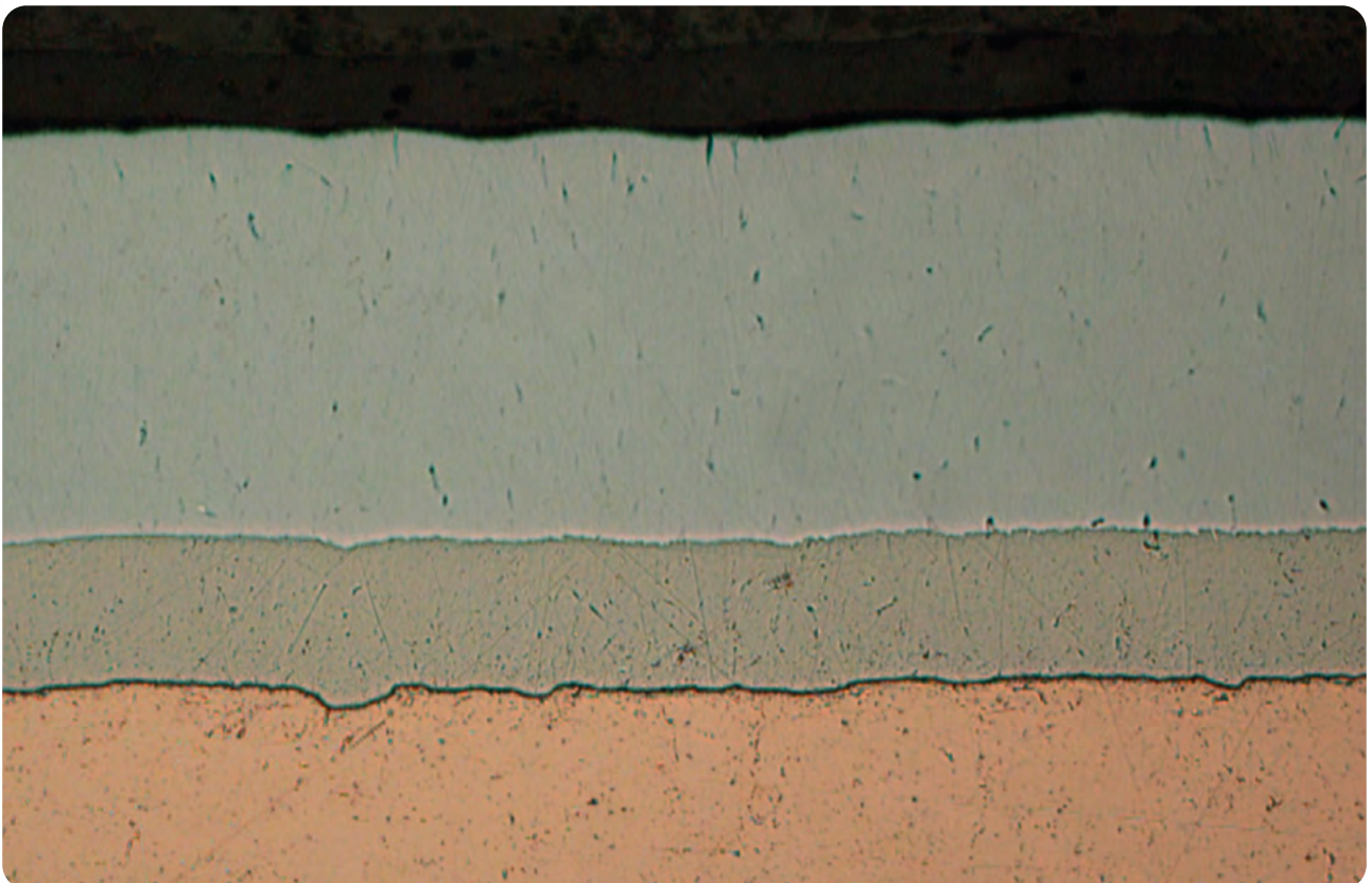
Sectional view of the AMC®-ML coating in the ingot mould tube
