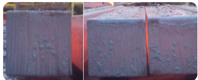
WAVE Mould billet (left) with excellent shape compared to standard mould billets (right)
