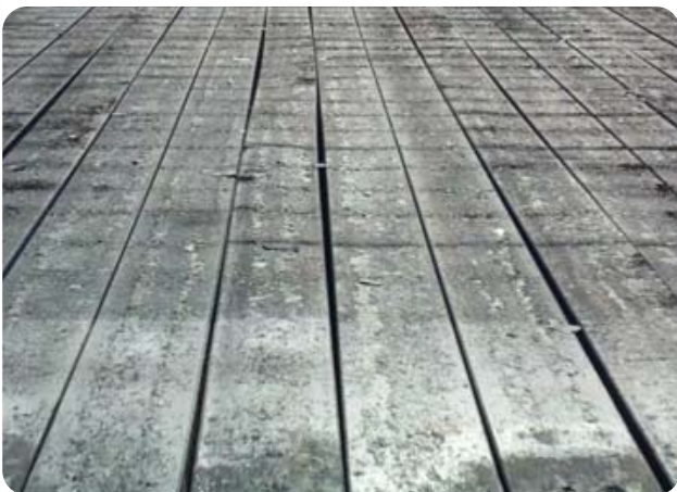
"Snaky" billets cast with standard moulds seen on the cooling bed
