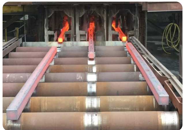
All three WAVE Mould strands in continuous operation
