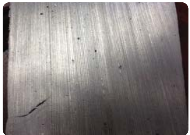
Off-corner hinge cracks from rhomboid billet shape
