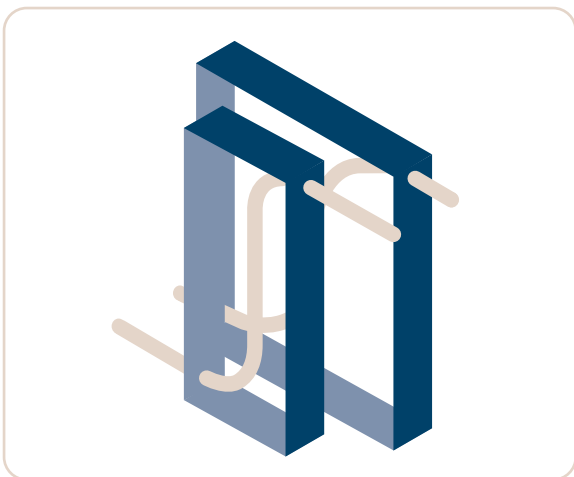
This figure shows the different needed space (grey border) of an S-curve bending of tube bundles.
